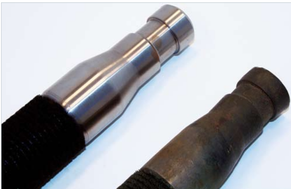
Left: New brush plunger Right: Brush plunger with flattened fishing neck from excessive impact.
