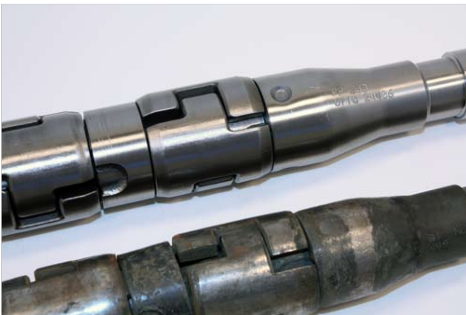
Top: New double-pad plunger Bottom: Double-pad plunger with pad shoulders worn down.
