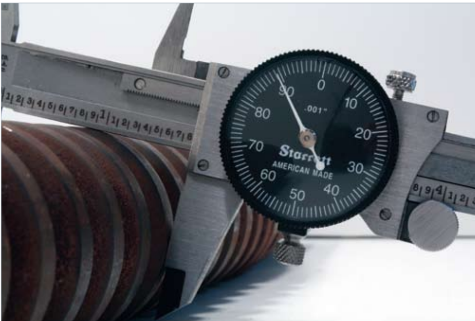
Calipers on Flow-Thru plunger measures outer diameter.
