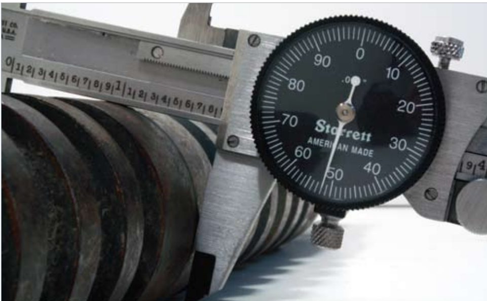
Calipers on solid plunger measures outer diameter.
