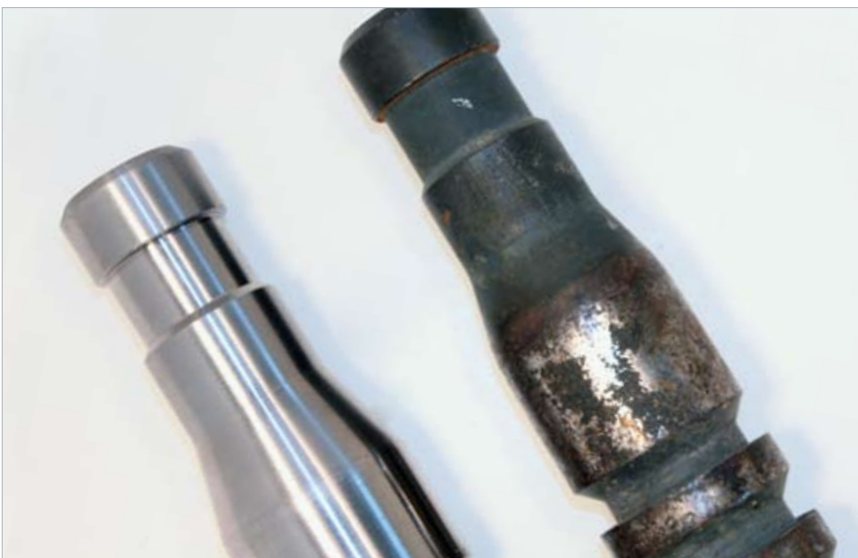
Left: New solid plunger Right: Solid plunger with visible corrosion and fishing neck compression.
