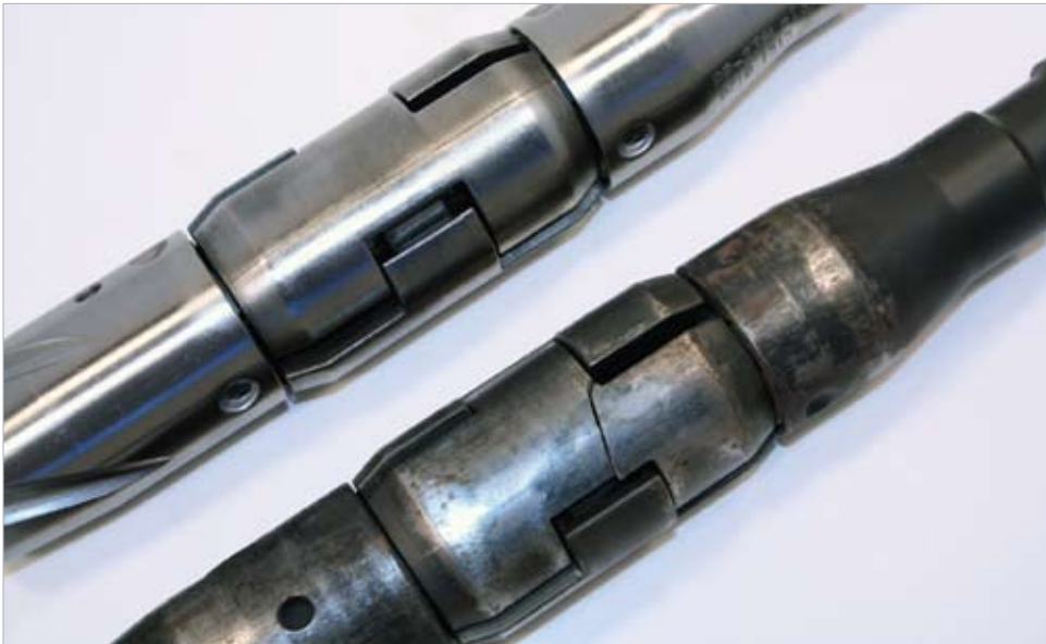
Top: New Liquid Aeration Plunger™ Bottom: Liquid Aeration Plunger™ with a crack in the pad.
