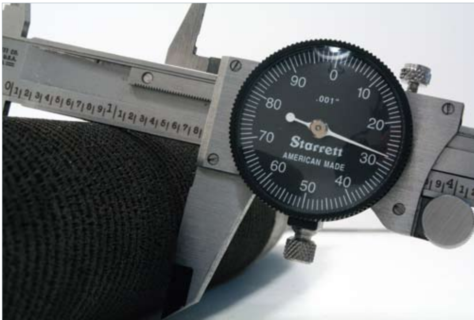
Calipers on brush plunger measures outer diameter.
