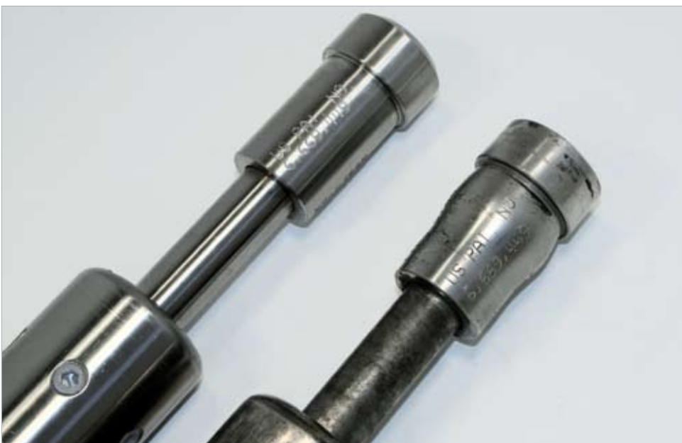
Left: New Flow-Thru Plunger Right: Flow-Thru Plunger with swollen fishing neck from excessive impact.
